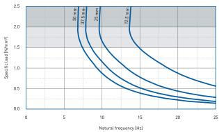
Natural frequency of a single-degree-of-freedom system consisting of a fixed mass and an elastic bearing consisting of VIKADYN VD 1500 on a stiff subgrade.
