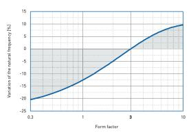
Correction values varying form factors specific load 0.35 N/mm<sup>2</sup>. Form factor q = 3
