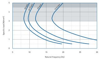
Natural frequency of a single-degree-of-freedom system consisting of a fixed mass and an elastic bearing consisting of VIKADYN VD 3000 on a stiff subgrade.
