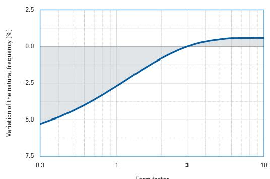
Correction values varying form factors specific load 0.15 N/mm².
