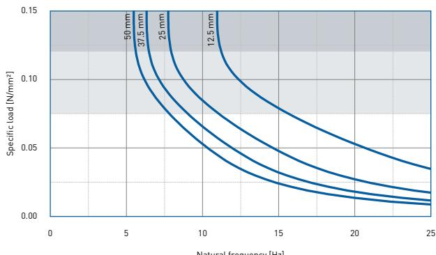
Natural frequency of a single-degree-of-freedom system consisting of a fixed mass and an elastic bearing consisting of VIKADYN VD 150 on a stiff subgrade.
