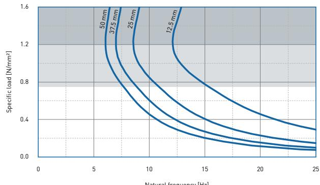
Natural frequency of a single-degree-of-freedom system consisting of a fixed mass and an elastic bearing consisting of VIKADYN VD 750 on a stiff subgrade.
